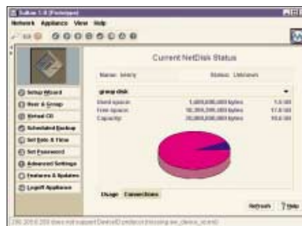
When the user clicks on Connect, ApplianceView asks the appliance for the latest configuration files, then brings up the admin screen for the selected appliance.
